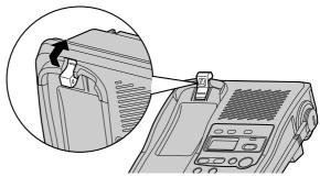
Press the tabs in the direction of the arrows (1), then remove the wall mounting adaptor (2).
