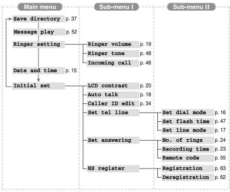
•If you program the date and time, the dialing mode, the flash time, the line mode, the number of rings, the recording time or the remote code using one of the handsets, you will not need to program the same function using the other handsets.
